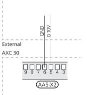
At 0 V the shunt is closed and at 10 V the shunt is open.
