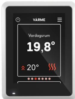
The NIBE RMU S40 is a wireless\*/wired room unit with a 2.8" touch screen and built -in temperature and humidity sensors. You use it for remote control and monitoring of your NIBE S series heat pump, as a supplement to the myUplink app in your smartphone or tablet. The room unit is easy to position and simple to use with an intuitive interface. The room unit also enhances the signal between your smart home products when these are located at a distance from each other.
